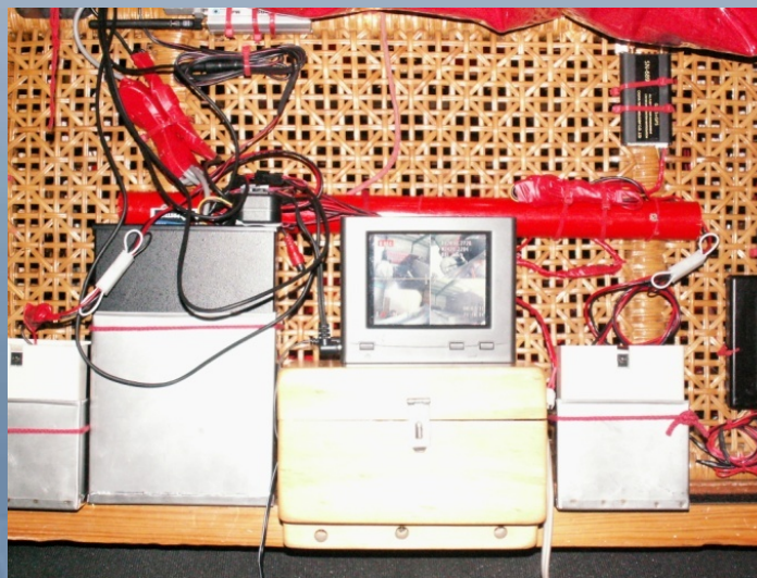
The DVR and the batteries installed at the back of the sedan chair.
